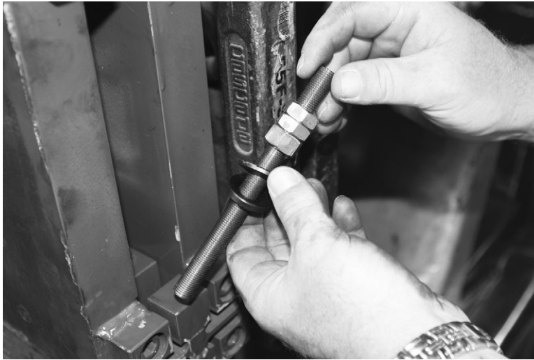
Figure 6-80. Install Spherical Washer Set
