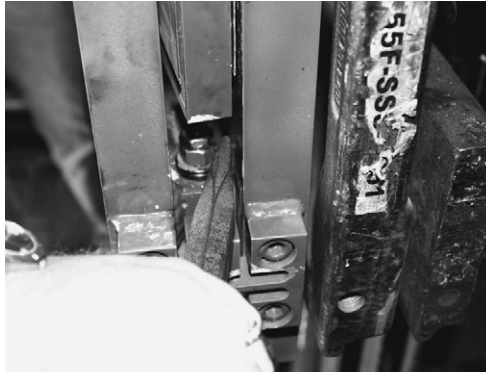
Figure 6-82. Centering the Load Cell Using a Chisel
