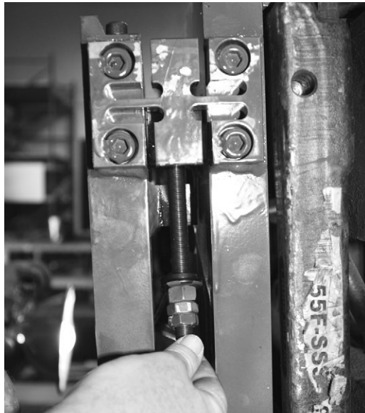
Figure 6-78. Installing Flexure into Scale
