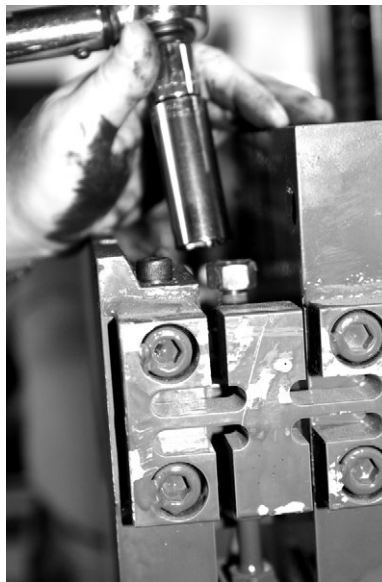
Figure 6-72. Removal of Hex Nut (#1 of Parts Breakdown)
