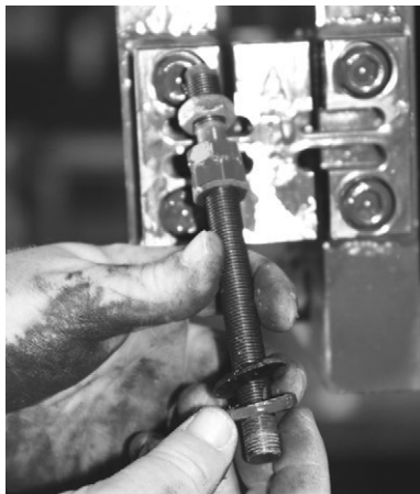
Figure 6-74. Remove Flexure Rod with Nuts and Washers
