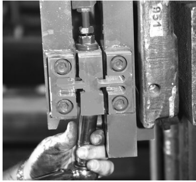
Figure 6-73. Loosen and Remove Bottom Hex Nut (#18 and #19 on Parts Breakdown)
