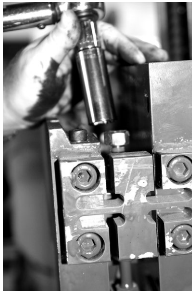
Figure 6-3. Removal of Hex Nut (#1 of Parts Breakdown)
