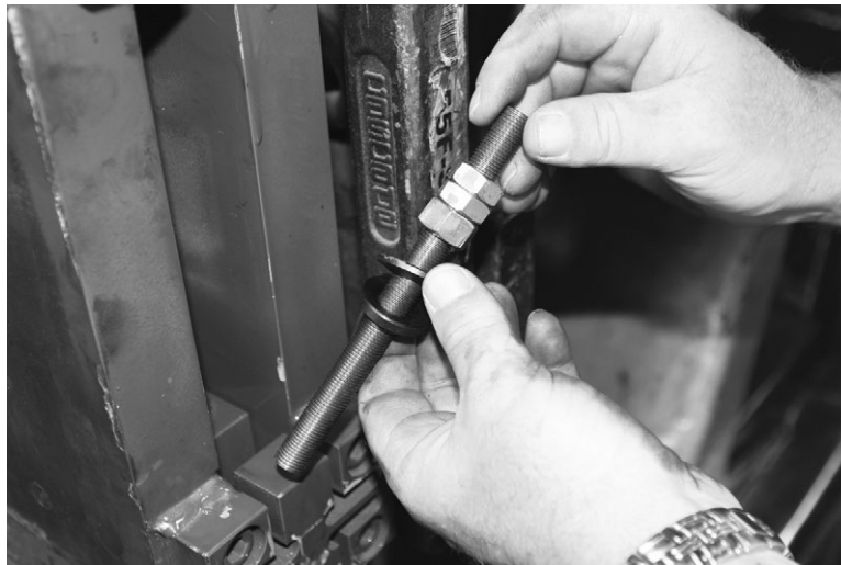
Figure 6-10. Install Spherical Washer Set
