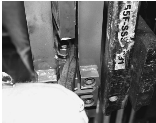
Figure 6-12. Centering the Load Cell Using a Chisel
