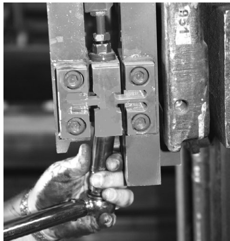
Figure 6-13. Tightening the Lower Hex Nut
