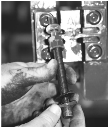
Figure 6-5. Remove Flexure Rod with Nuts and Washers
