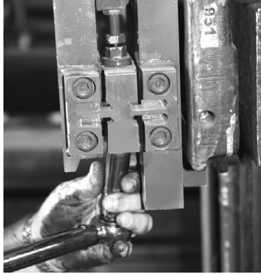
Figure 6-4. Loosen and Remove Bottom Hex Nut (#18 and #19 on Parts Breakdown)
