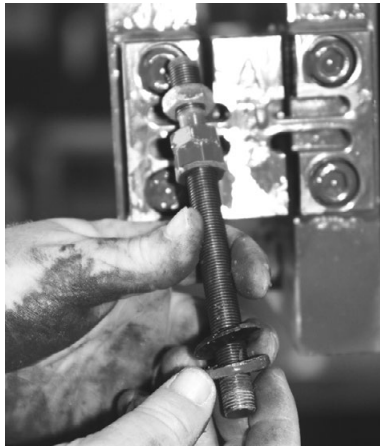
Figure 6-5. Remove Flexure Rod with Nuts and Washers
