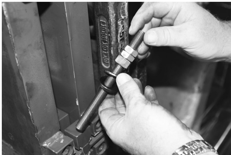
Figure 6-10. Install Spherical Washer Set
