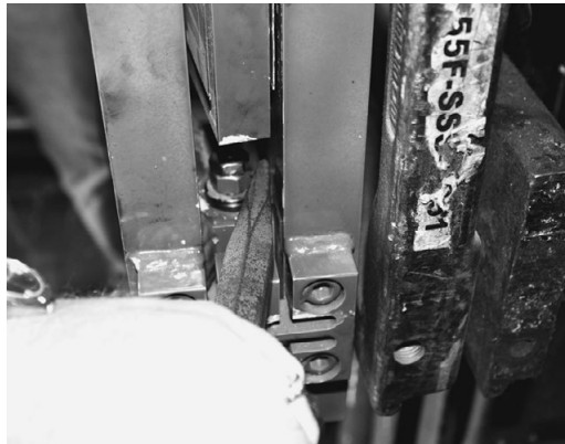
Figure 6-12. Centering the Load Cell Using a Chisel
