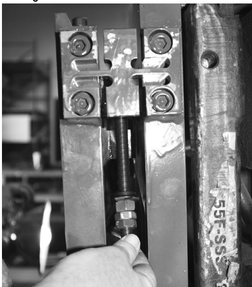
Figure 6-8. Installing Flexure into Scale
