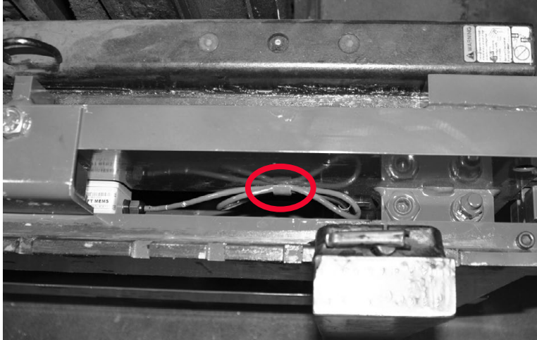
Figure 6-6. Load Cell Cable Clips
