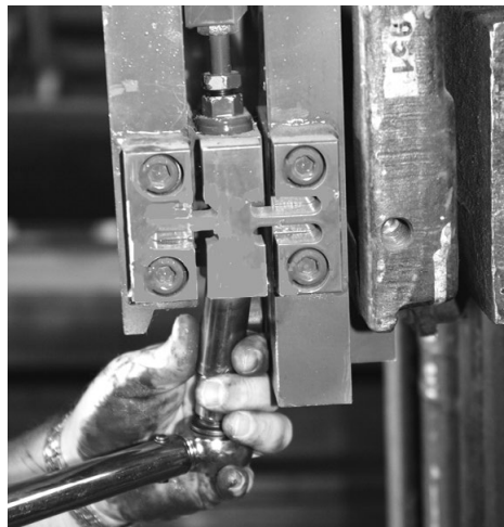
Figure 6-13. Tightening the Lower Hex Nut
