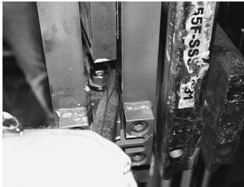
Figure 6-13. Centering the Load Cell Using a Chisel
