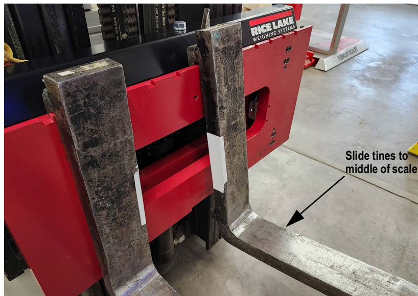
Figure 7-1. Forklift Tine Removal
