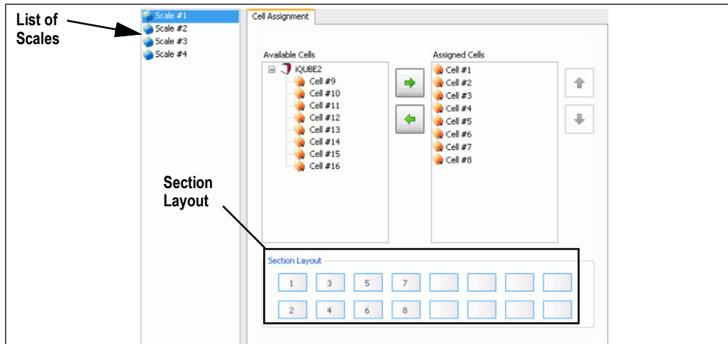
Figure 5-6. iQUBE 2 Section, Load Cell Assignment
