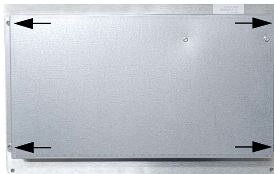
Figure 7. Ai-1 Indicator Cover Mounting Bolts
