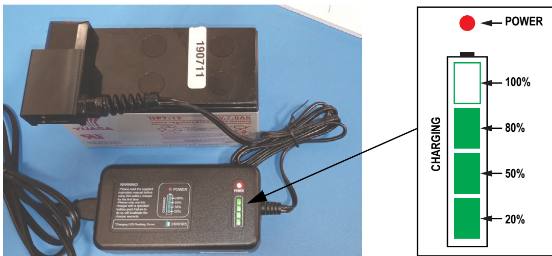
Figure 2-1. Battery Charger Connected to Battery
